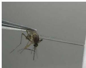
Figure 3: Dose being directly applied to mosquito using capillary action micropipette.
