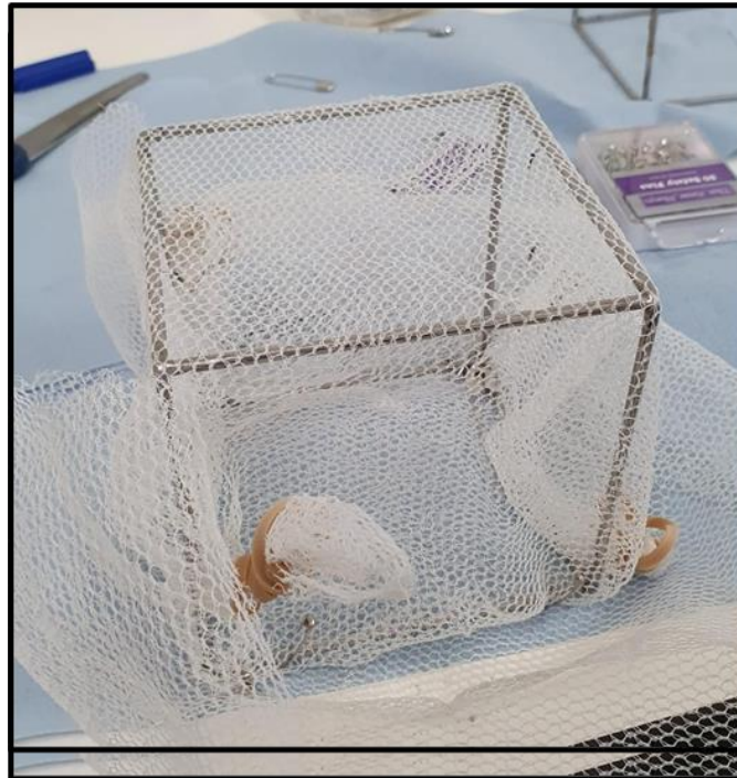
Figure 1.. Image of cube variant of WHO wire ball assay in use. The image shows netting material wrapped around the metal cube frame and secured in place with elastic bands.
