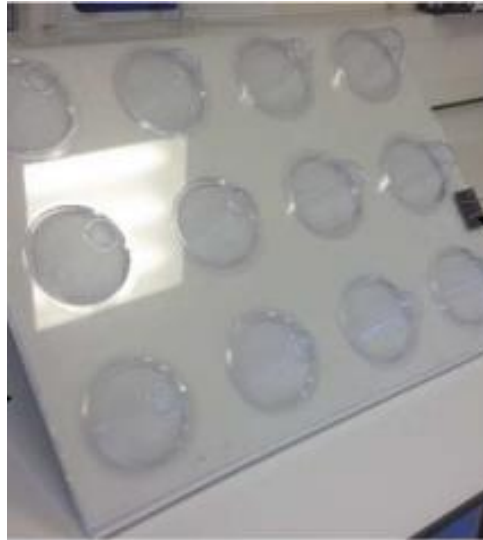
Figure 1: Set up of a standard WHO cone test board. Image from LITSOP007.
